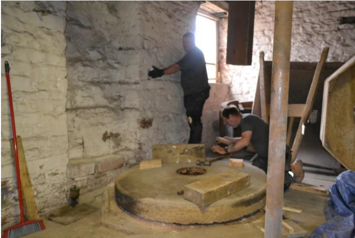
Figure 1 lifting the runner stone with levers and wedges to clean the oat stones
