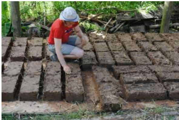
Drying the blocks on a flat surface
